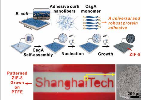
Figure 2. MOF crystals (red) grown on various polymeric substrates with different morphologies
